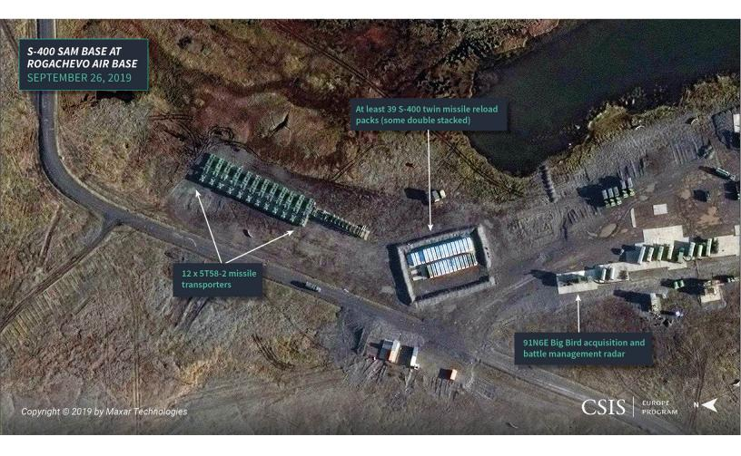
and battle management radar, a LEMZ 96L6-1/96L6E acquisition radar, two 5P85SM/SE2 self-propelled transporter erector-launchers (likely as spares or for training), and a number of support vehicles and trailers.
