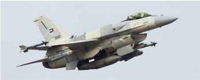
The F-16E/F Block 60, operated only by the UAE, is more advanced than the F-16C/D Block 50s of the U.S. Air Force. Source: [F-16.net](http://F-16.net)
