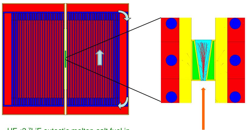
UF<sub>4</sub>:2 <sup>7</sup>LiF eutectic molten-salt fuel in graphite matrix; rapid circulation between core and internal primary heat exchanger; continuous low-volume feed-and-overflow permits equilibrium operation
