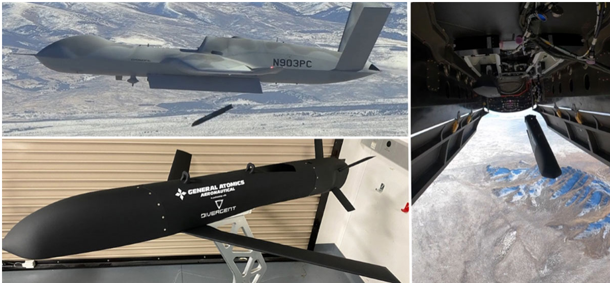
Figure 8: General Atomics' A2LE Launches from MQ-20 Avenger UAS
