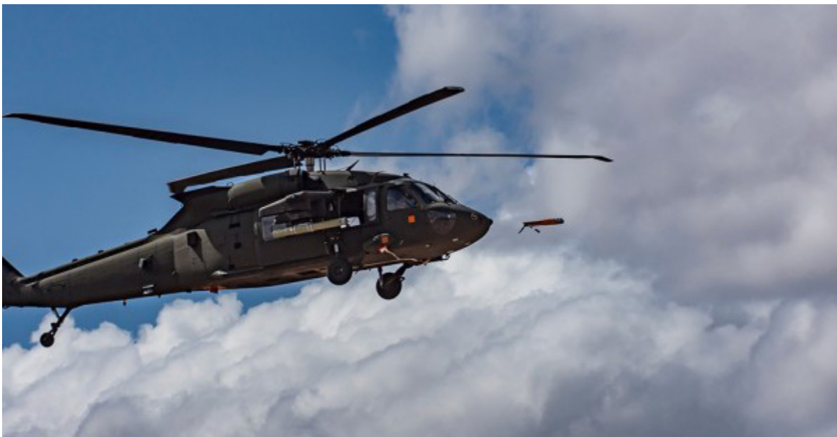
Figure 13: Launch of an ALTIUS-600 by UH-60 Black Hawk Helicopter
