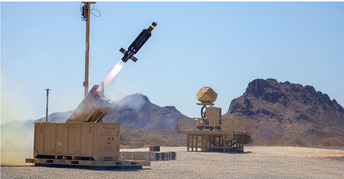
Figure 11: Raytheon’s Coyote Block 2 (Kinetic C-UAS Effector) Launching from the U.S. Army’s Low, Slow, Small Unmanned Aircraft Integrated Defeat System (LIDS)
