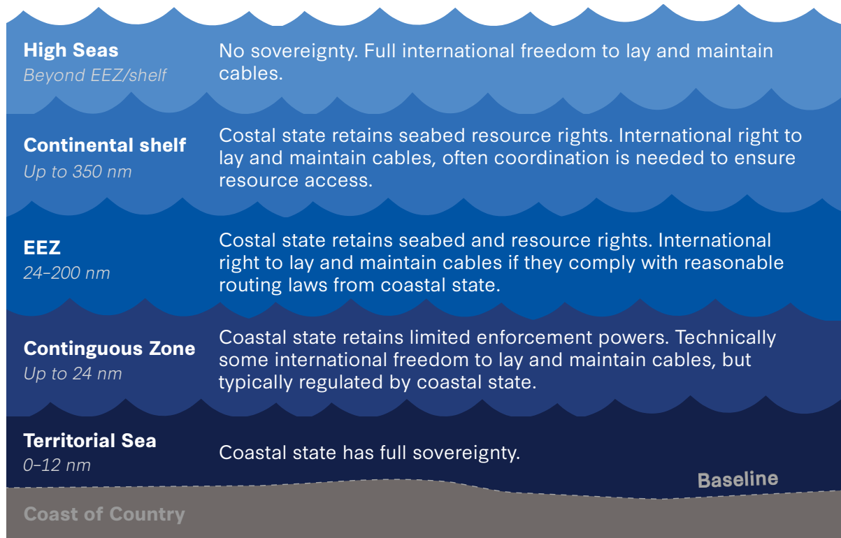
Figure 7: Maritime Zoning Rules for Subsea Cables per UNCLOS
