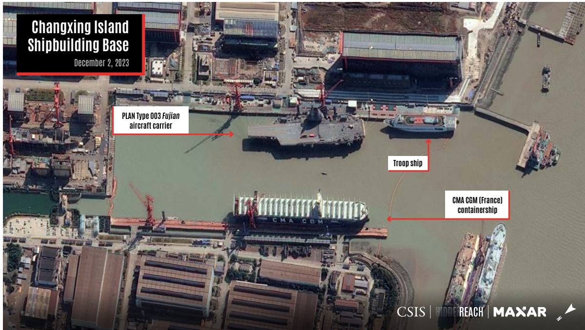
Figure 10: PLAN Warships Built Alongside Merchant Vessels at Tier-1 Shipyards (See Appendix for Additional Imagery)
