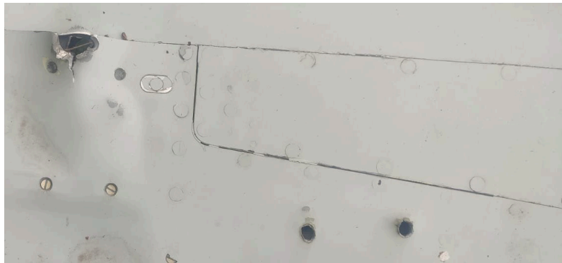
Damage from air defense interceptor on body of downed 3M-14 Kalibr cruise missile, June 2022.
